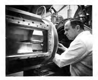
TEST CHAMBER downstream from new Mach 14 wind tunnel nozzle is 18 inches in diameter, 33 inches in length. Don MacKenzie (5622) mounts a model of a Sandhawk instrumentation rocket for a test run.
